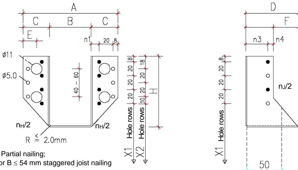
Drawing: Blank 280, 2.0 mm steel    Type short: reduced bottom plate
