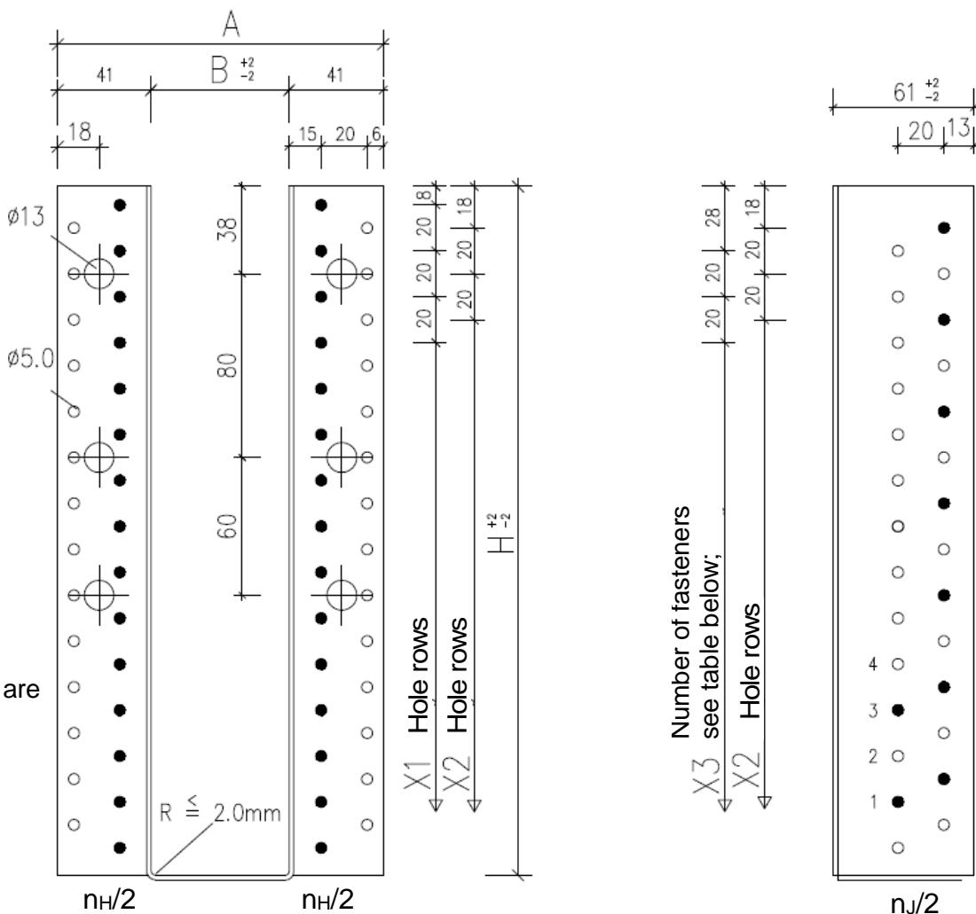
Height interval: 160 mm – 320 mm; Width interval: 100 mm – 240 mm; Joist hanger's height = (blank – width)/2
