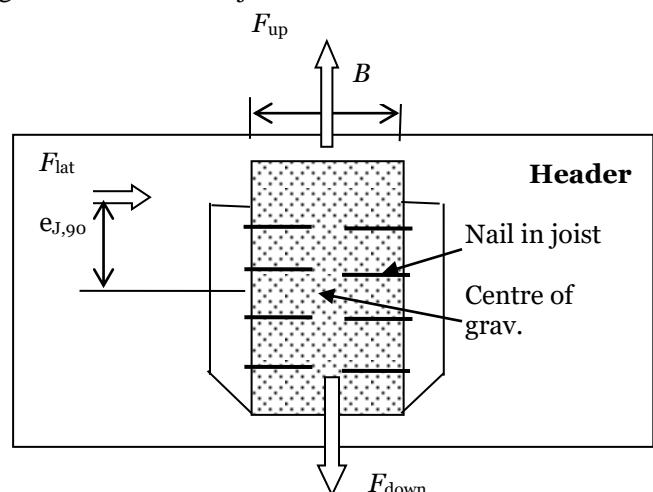
It is assumed that the header beam is prevented from rotating. Similarly, it is assumed that the concrete structure or the steel member to which the joist hanger is bolted does not rotate. If the header beam only has
