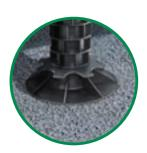
To make sure that the substructure does not come into direct contact with damp soil or stones, it is mounted on evenly spaced concrete slabs. To improve ventilation from below, at least one SPAX Pad should be inserted between the substructure and concrete slabs. Or, even better, use SPAX Lift adjustable feet for easier levelling of the decking surface.
